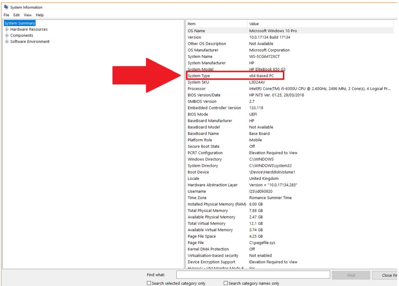
The screenshot shows the 'System Information' window with the 'System Summary' tab selected. A red arrow points to the 'System Type' entry, which is highlighted with a red box and shows 'x64-based PC'.
